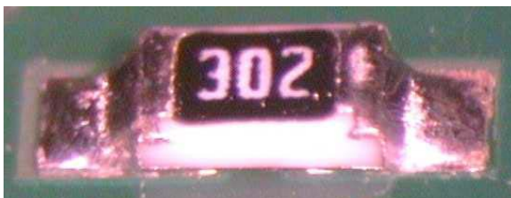
Well soldered SMD bottom-side
