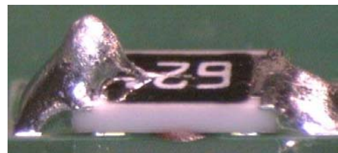
Icicling of SMD using No-clean ROLO Flux
