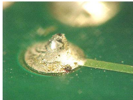
Higher temperature pot 275°C
