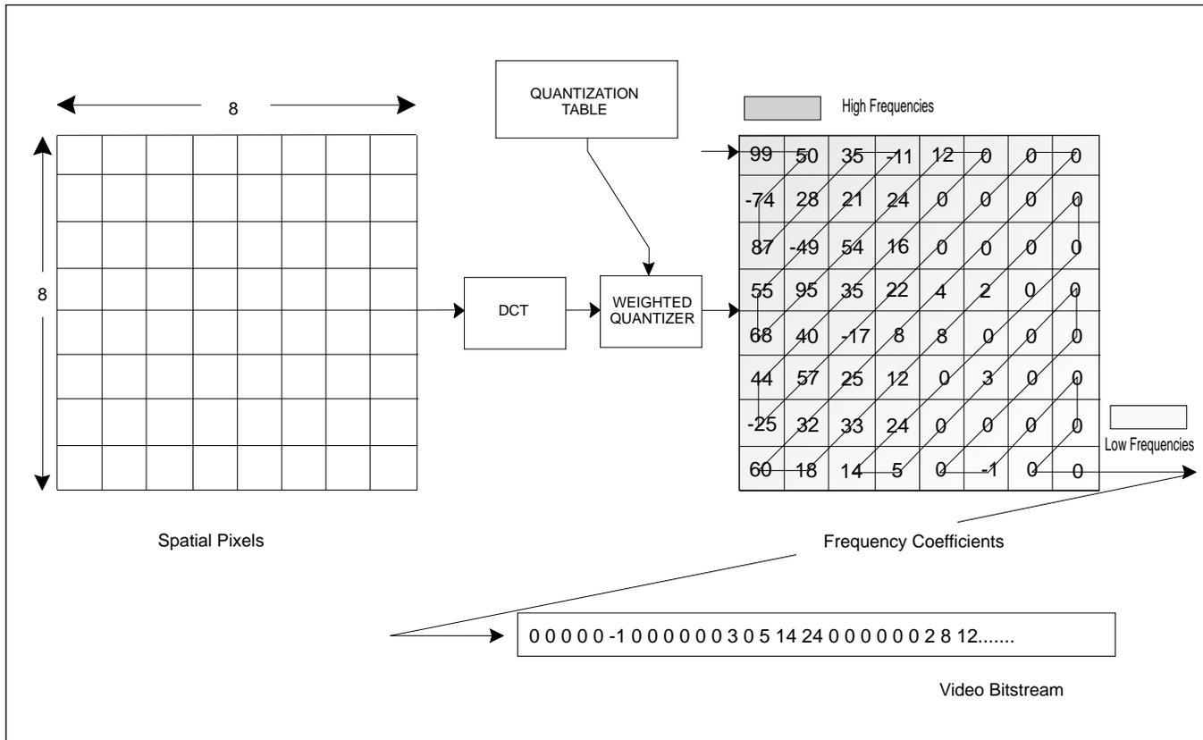
Figure 8. DCT coding and quantization (numbers are hypothetical).
